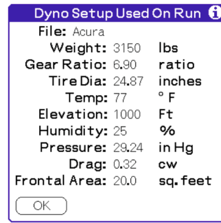
Figure 39: Menu “Dyno Setup Used On Run”
